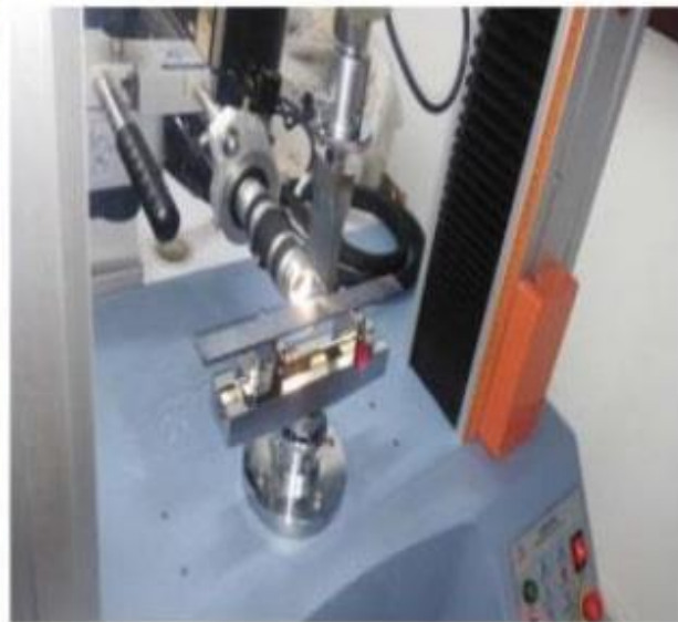
(b) Three-point bending
